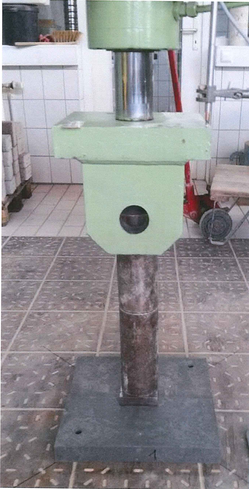
Figure 1: Load test with rigid support
