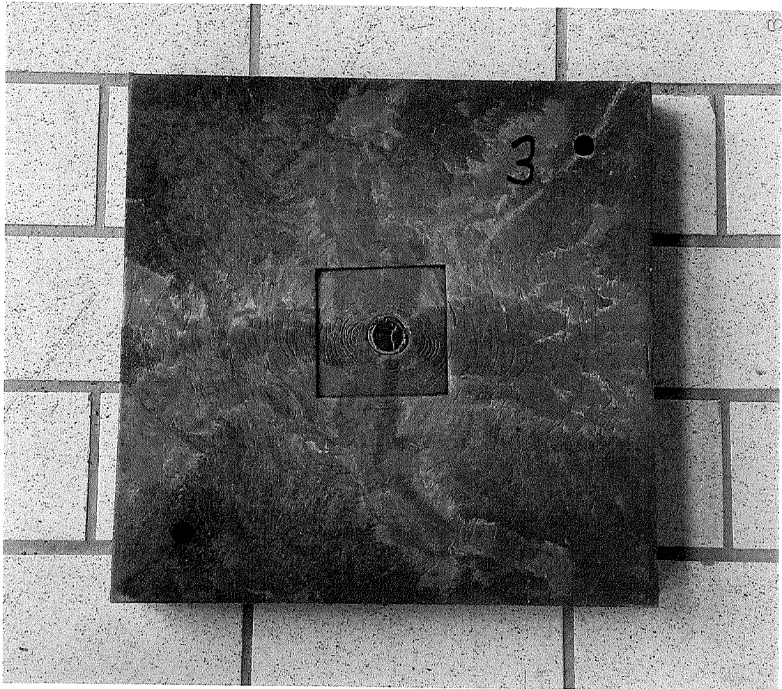
Figure 3: Plastic slab, thickness 50 mm, following the test on rigid support. Clearly visible: indentation of the load slab in the middle of the tested piece.
